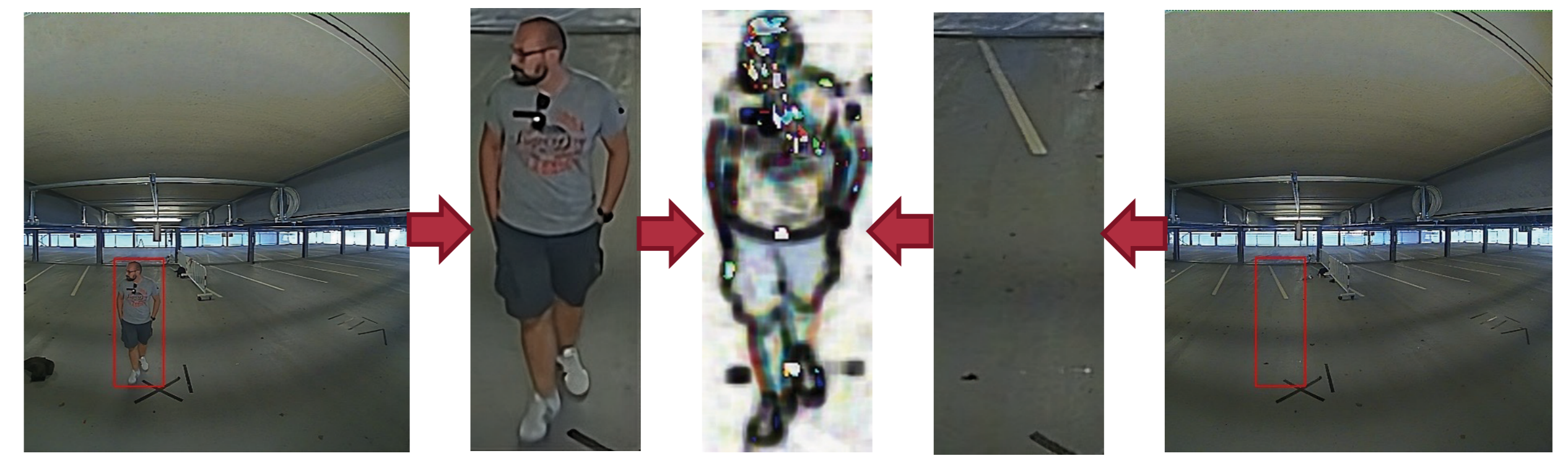
Figure 4: Detection in the camera image (left), the same corresponding empty image (right) and the difference of the cutout calculated with the structural similarity (SSIM).
